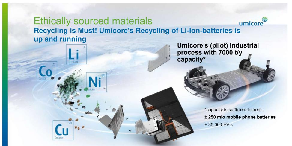
Umicore combines Pyro & Hydro technology to recycle and refine the module → Metals are recovered in battery grade quality! Materialinnovationen für die Dekarbonisierung des Verkehrs, Umicore, Dr. Paul Spurk
